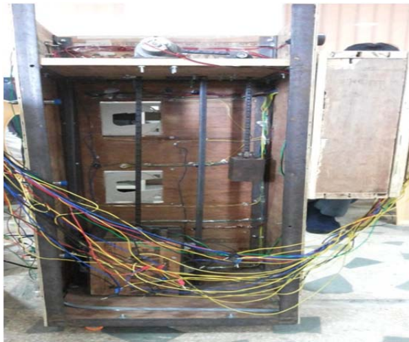
Fig. 4: model of elevator control(Back side)
